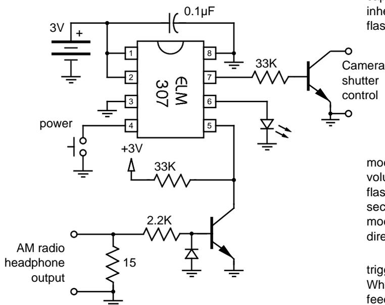
Figure 2. Lightning Detector
